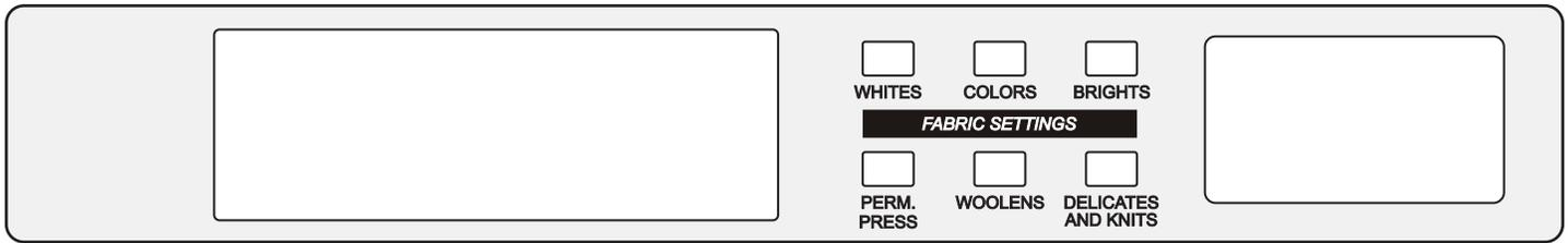
**NOTE:** After the washer has been installed and plugged in, the display will show '0 MINUTES'. Once the washer has been plugged in and the washer door opened and closed, the display will show the price. In washers set for free cycles, the display will flash 'SELECT CYCLE'.
